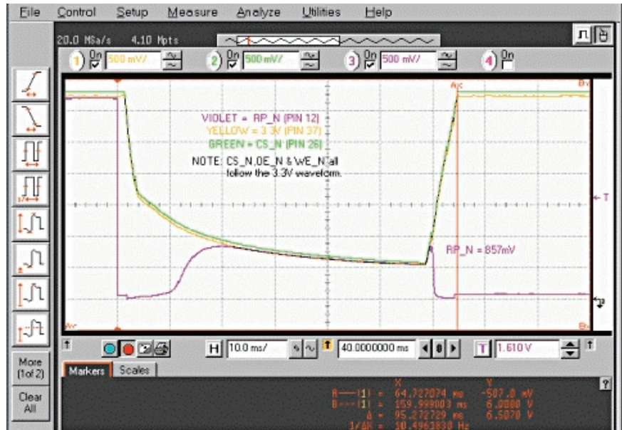
Figure 6. With a temporary capacitor added to prevent the 3.3 V from dropping into a range that sent the memory module into an indeterminate state, the module began generating valid data.
